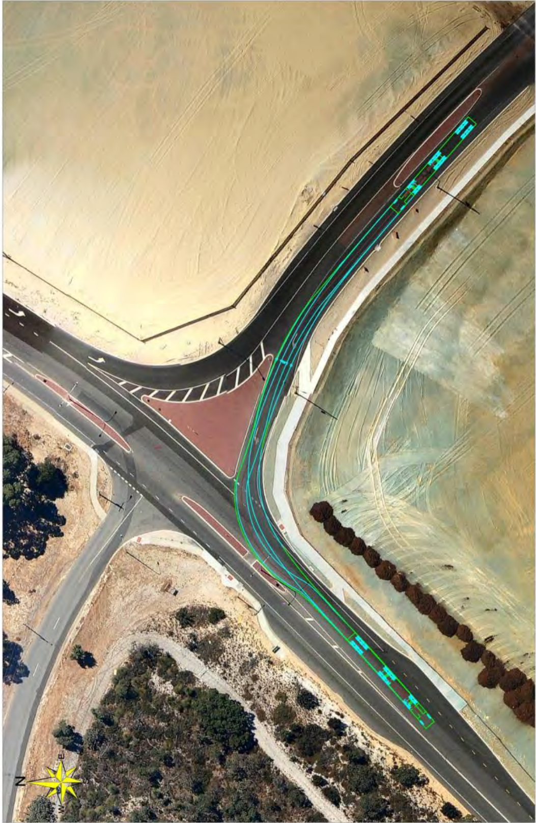
Proposed K-Mart Distribution Centre, Jandakot 27.5m B-Double Truck Turnpath Assessment : Left Turn from Spartan Street into Berrigan Drive
