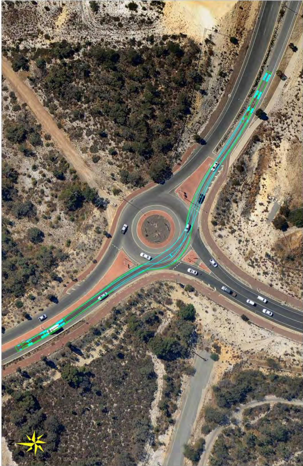
Proposed K-Mart Distribution Centre, Jandakot 27.5m B-Double Truck Turnpath Assessment : Karel Avenue and Berrigan Drive Roundabout - Through Movement Westbound along Karel Avenue
