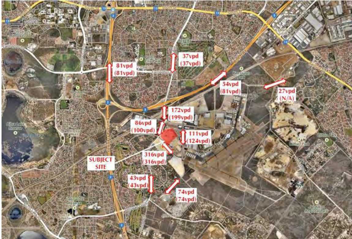
Figure 3. Estimated typical weekday traffic generated from the proposed development – assessment year 2031 (interim scenario year 2016/2018)
